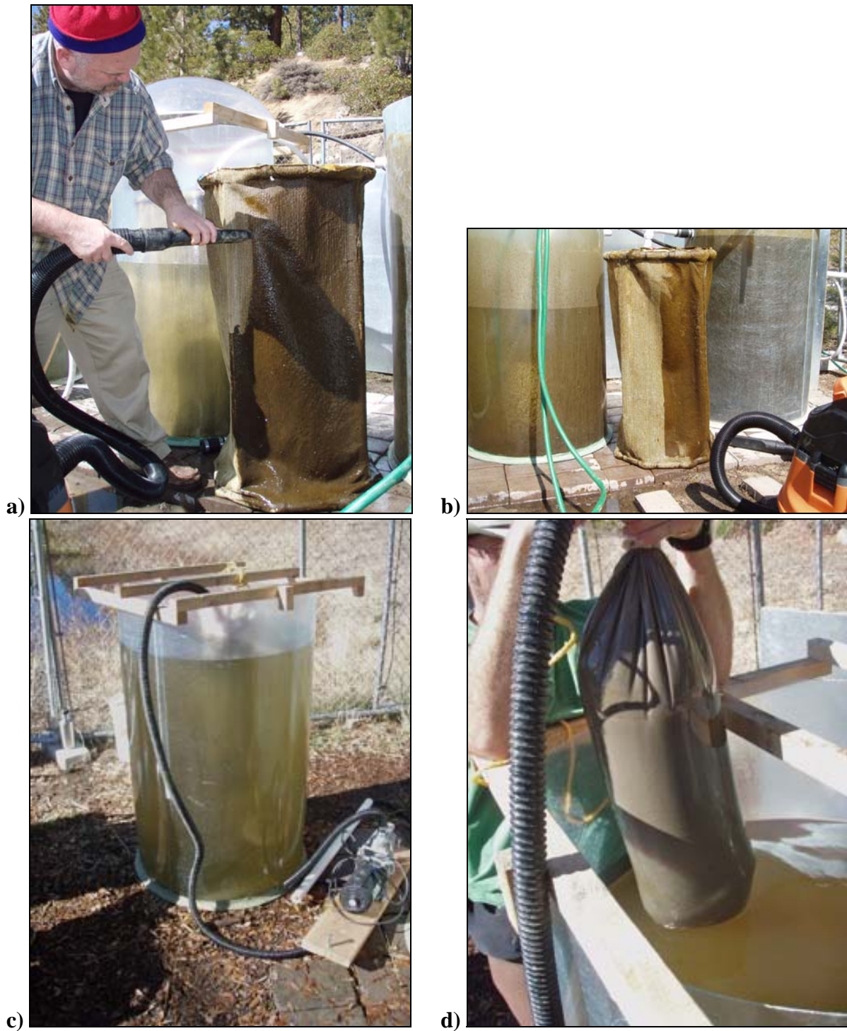
Figure 8. Periphyton harvesting sequence: a) and b) vacuuming biofilm from screen, c) and d) pumping tank water through filter to capture dislodged periphyton.
