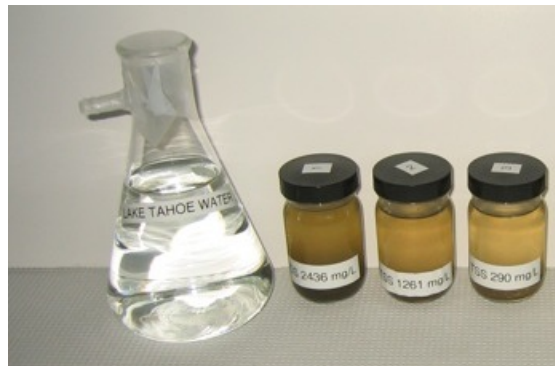
Pristine Lake Tahoe water on left vs. polluted urban stormwater on right (Source: A. Heyvaert).
